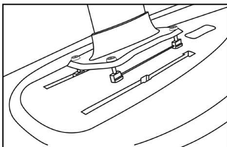
2 Insert the SCS inserts over the holes in the carbon plate.
