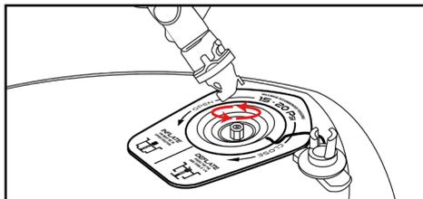
Before proceeding with your first inflation, tighten the valve with the black key that comes in the repair kit to insure perfect functioning (**instructions in WARNING**).
