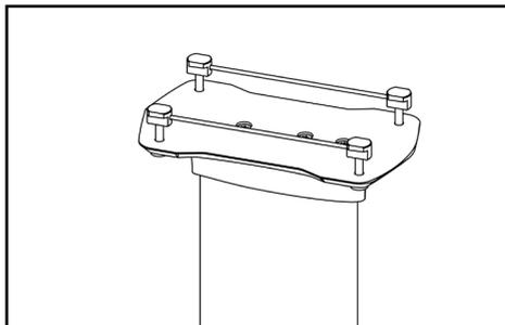
1 Place your foil on a smooth surface. Install the two SCS inserts with the recommended screws.
