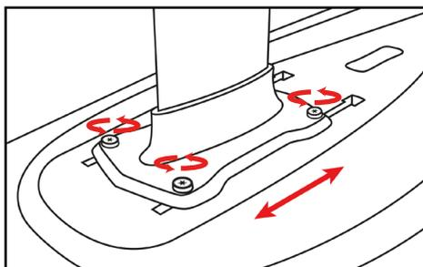
3 Slide your foil to the desired setting. Tighten all screws. **Your board is ready for use.**
