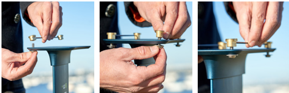
1 Place your foil on a smooth surface. Install the two SCS inserts with the recommended screws.
