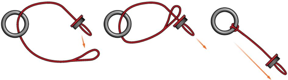
Reassemble your kite leash and then connect your kite leash to the safety ring on the bar before launching your kite. To access the carabiner, slide the foam protection downward. Clip the carabiner onto the ring in the middle of the chicken loop. Fold the foam protection back over the carabiner.
