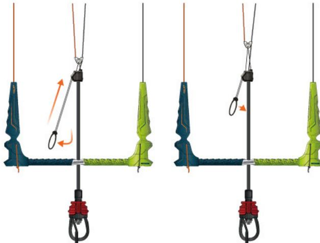
To lengthen them, grab the trim handle and pull gently towards you to unlock the end from the cleat. Release it gradually until the desired position, then secure the end back into the cleat.
