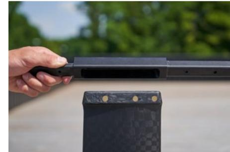
**1** Connect the mast to the fuselage with the 3 **M6-50 mm** screws **D**. The thickest part of the mast must face towards the square section of the fuselage.
