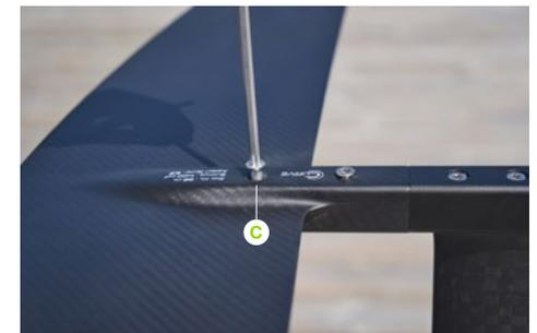
**2** First use the **M6-20 mm** **C** screw under the front wing. Tighten firmly.
