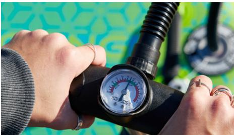
5 - Inflate to the required pressure which should be between **15 and 20 PSI**. It is normal to hear a small whistling of air at the Pump hose during inflation. Indeed, the tightness of the pipe is never perfect, but the losses are insignificant. Likewise, **the Pressure Gauge needle will only begin to move when the internal pressure of the board exceeds 5 PSI** : it is therefore normal that
