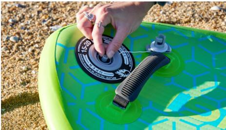
3 - **Make sure the Valve knob is in the up position for the inflation phase.** Just press the button and turn it to the right or left. If you do not follow this recommendation, the board will deflate when removing the hose from the valve.
