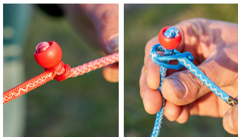
3 - Connect the Back Lines of the Bar to the Back Bridles of the Kite with an Larks Head Knot.
